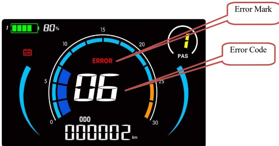
Example: In the above interface the error indicator shows **ERROR**, with the error code 06.
