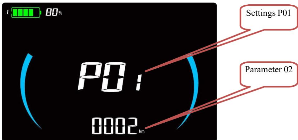
Example: In the above interface the setting item is **P01**, with the parameter value of **02**.
